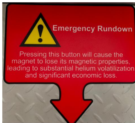
Fig4 Warning: Emergency Rundown
